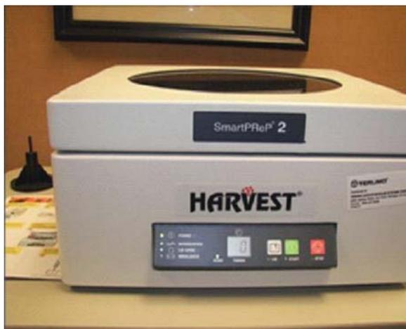
**FIGURE 1.** High velocity centrifuge provided by the vendor used in the separation process.
